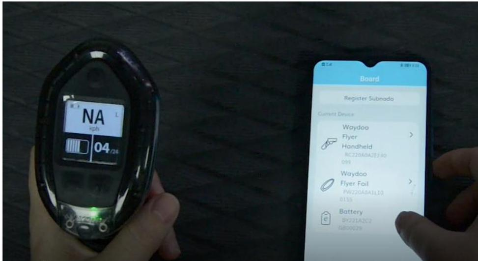
After the successful activation, three different parts will be displayed in the Current Device list on the Board page: Waydoo Flyer Handheld, Waydoo Flyer Foil, Battery, the device information will show the activation time.
