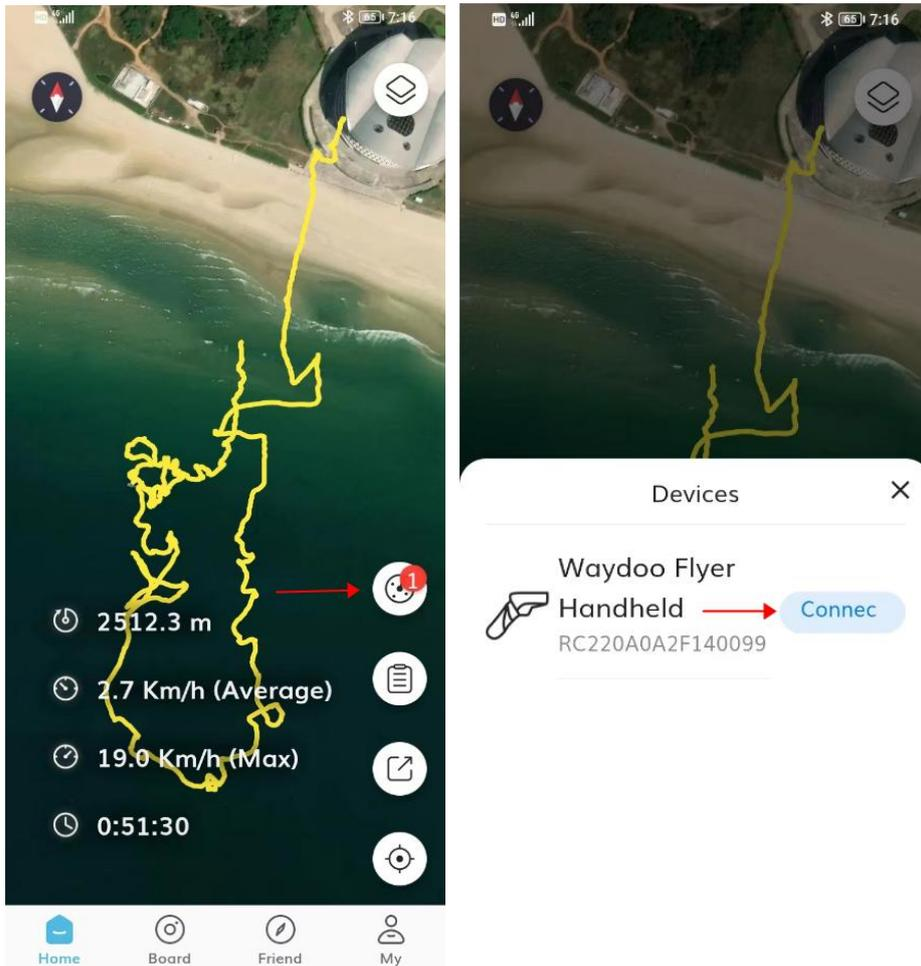
When the remote is first connected to Waydoo app, a four-digit verification code will pop up on the remote screen, please enter the verification code in Waydoo App within 15 seconds. After the verification code is entered correctly, the remote will be connected successfully, and prompts “Device Connected”.
