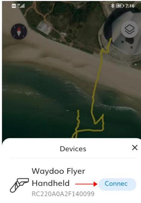
When the remote is first connected to Waydoo app, a four-digit verification code will pop up on the remote screen, please enter the verification code in Waydoo App within 15 seconds. After the verification code is entered correctly, the remote will be connected successfully, and prompts “Device Connected”.
