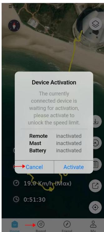
Enter the Board page, then click to expand the Device Information page, and click “Activate” button in the each page of Waydoo Flyer Handheld, Waydoo Flyer Foil, Battery to complete the activation of the three parts (as shown in the figures below).
